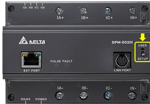
1. **USER mode:** If users know the setting of Modbus, they can communicate with the DPM-520I directly. Or users can set the settings of Modbus directly which they want.
