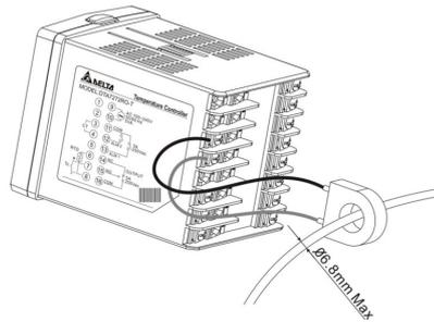
How to set up current input – remove the temperature controller cover and set JP8 to short. JP8 jumper locates near the sensor input area on PCB board.
